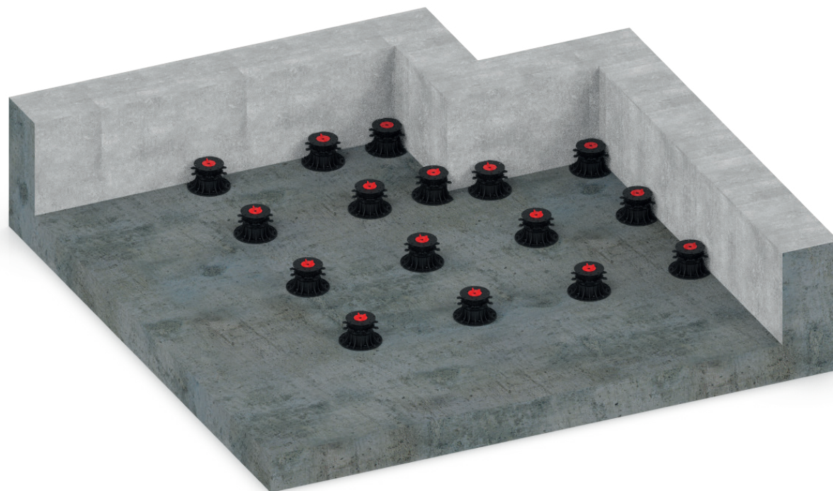
Example of pedestals placement
